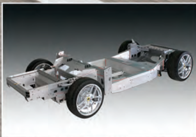
Exceptionally strong yet light weight epoxy-bonded extruded aluminum chassis.
